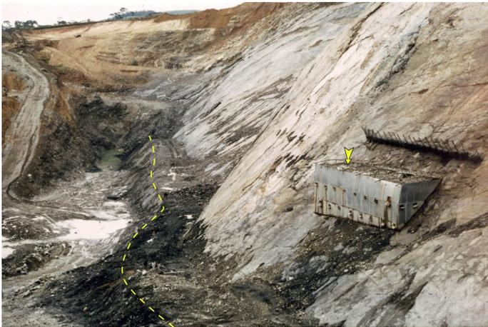
**Figure 4 | Same view after mining out reactor 2.** The metallic container pointed to by the yellow arrow hosts a slice of reactor 2 for further scientific studies. The top-left limit of the C1 layer ready for commercial exploitation is marked by a dashed line.
